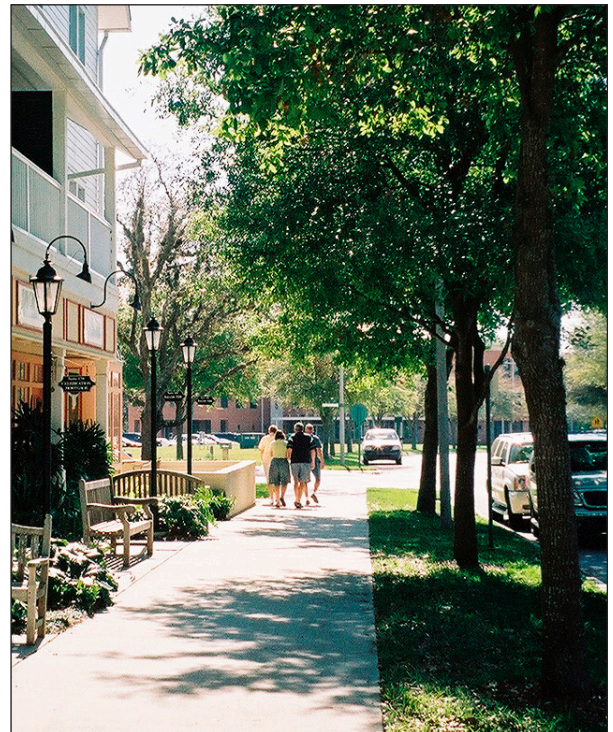
On-street parking, a planing strip and street trees provide the pedestrian a great buffer and sense of safety from passing vehicles.
