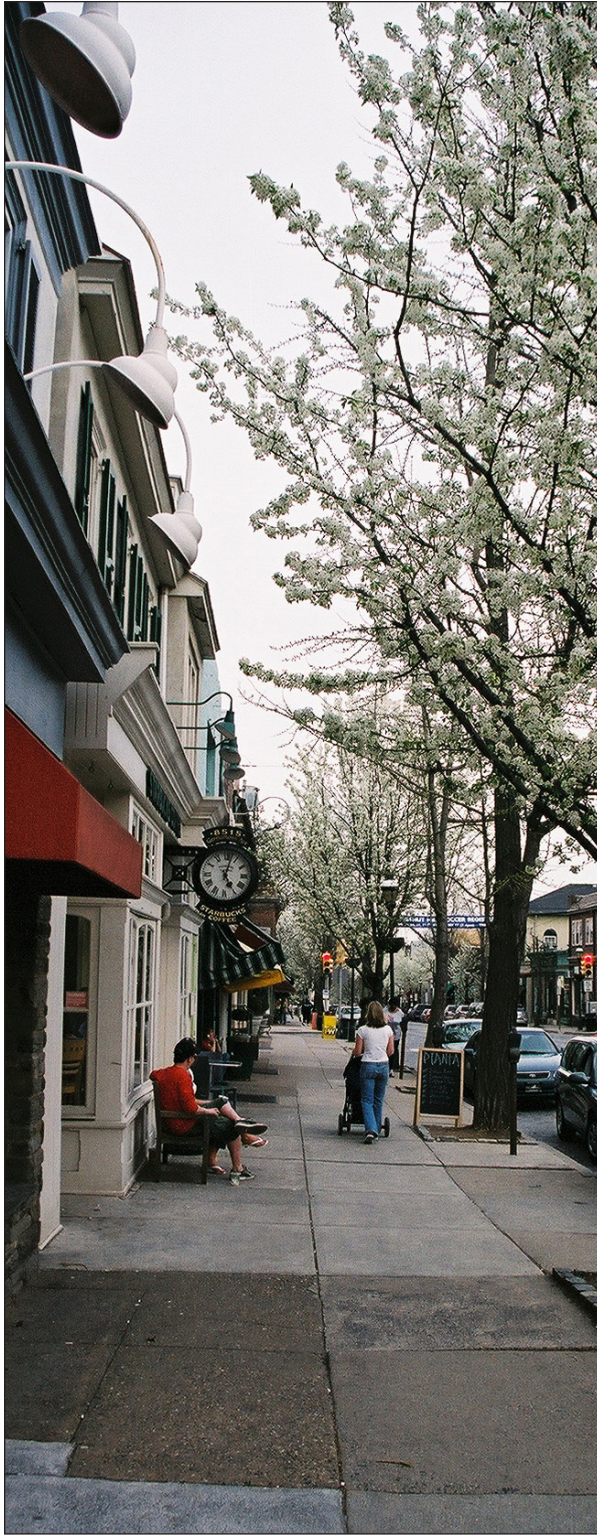
On this “main street” established towns often have the right sidewalk width, street trees, a number of places to sit and on-street parking to create a very usable and vibrant streetscape.
